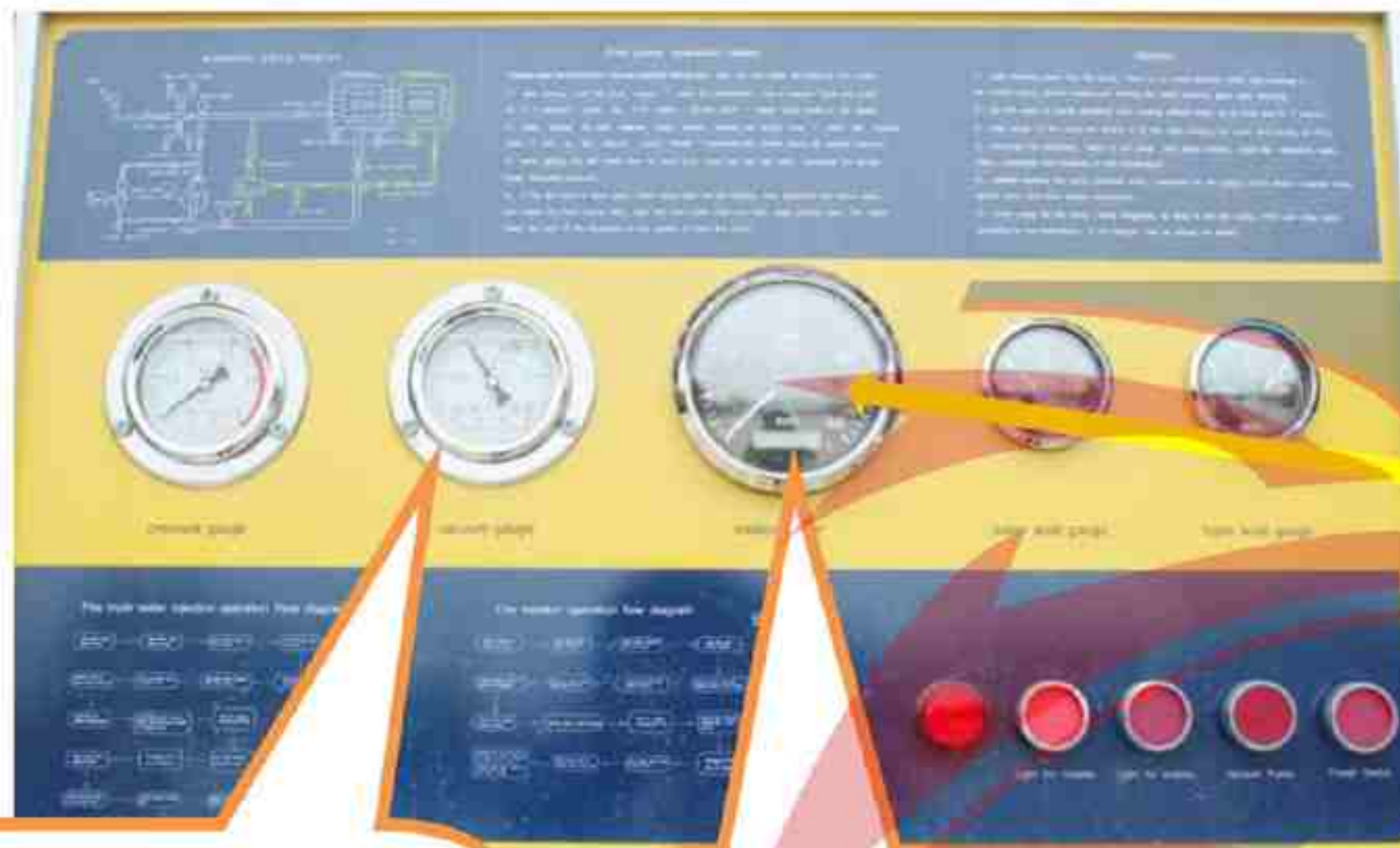
Vacuum Gauge at 0.02~0.04Mpa
