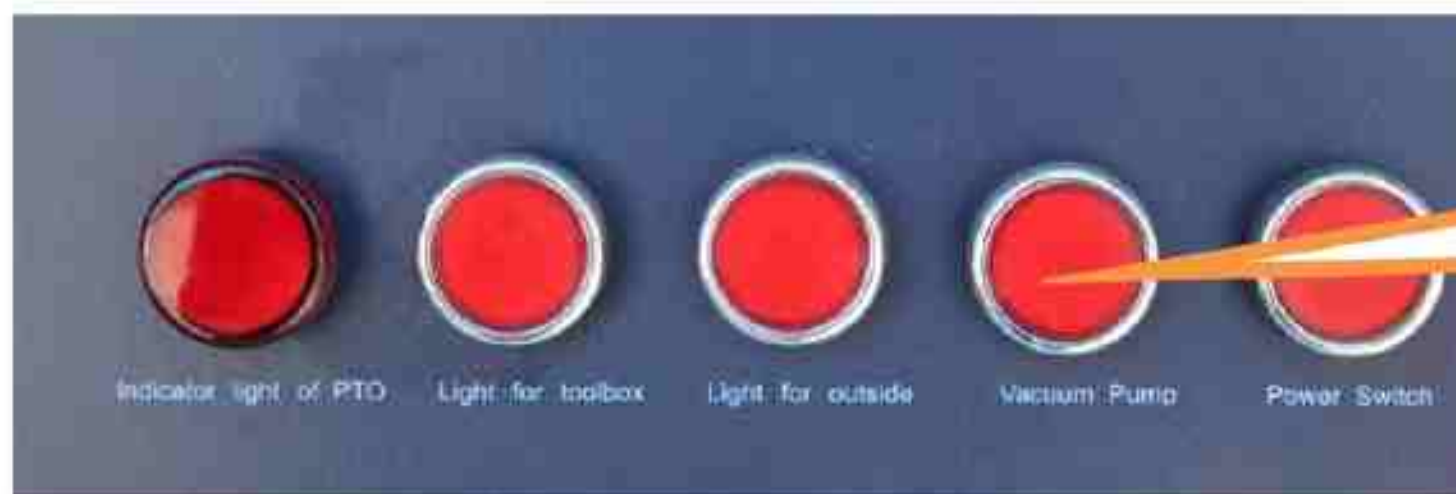
Press to turn off the main Vacuum Pump
